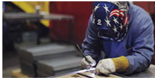
Electric Mirror welder at work on a luxury mirror metal frame to hold lighting and electrical components.
